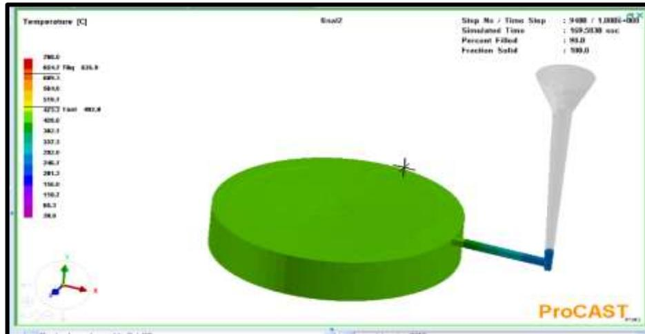
**Figure 3** Temperature variation of molten metal during pouring
