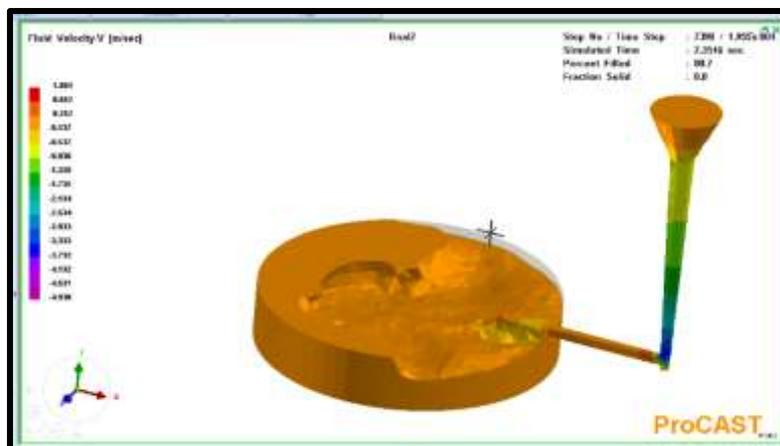
Figure 12 Fluid velocity in V-direction
