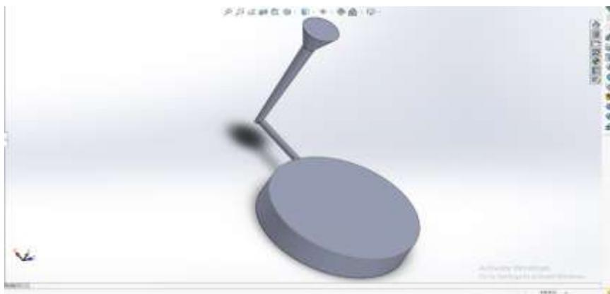
**Figure 2** Gear blank and Gating System Design
