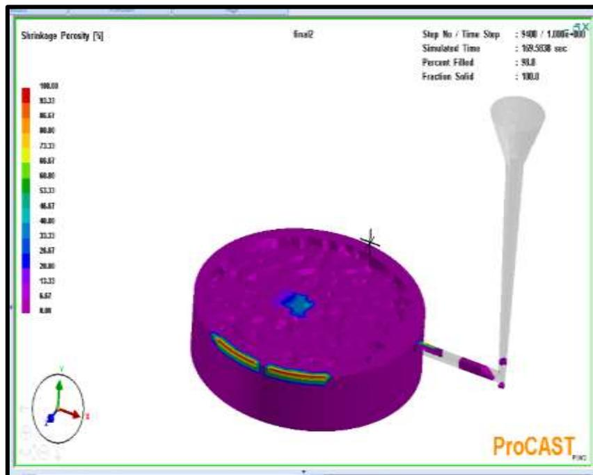
**Figure 6** Effect of Shrinkage Porosity
