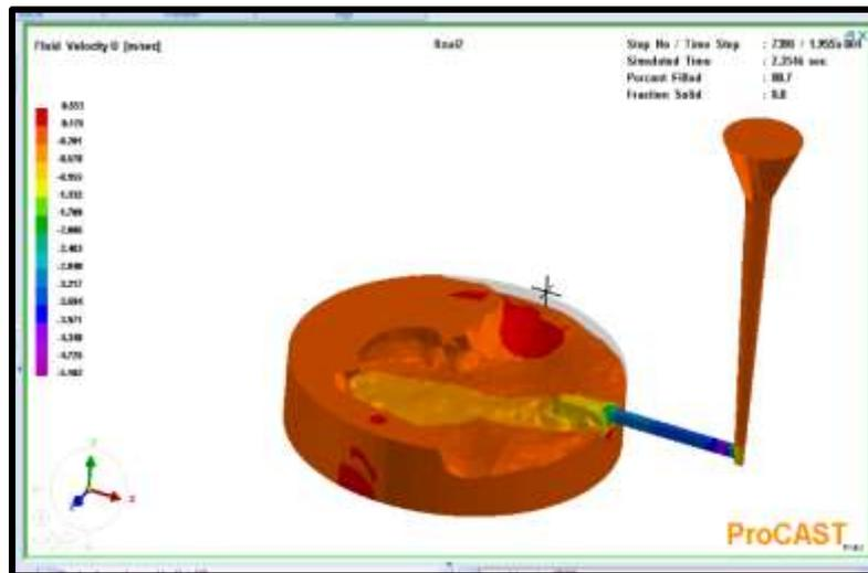
Figure 11 Fluid velocity in U-direction
