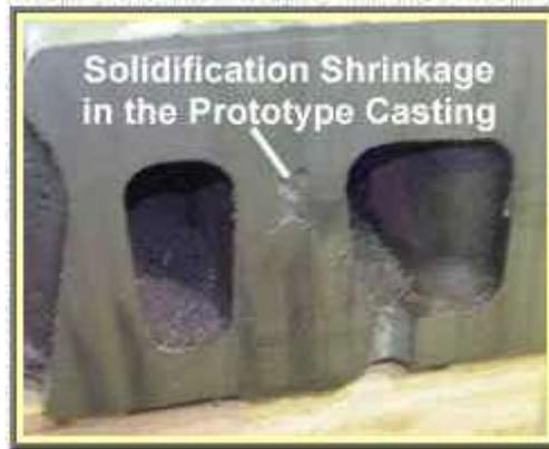
**Figure 1** Shrinkage and porosity [20]
