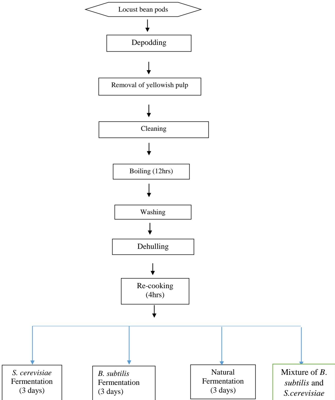
Fig. 1 - Flow diagram of traditional upgraded processing of locust bean seed to food condiment (Iru)
