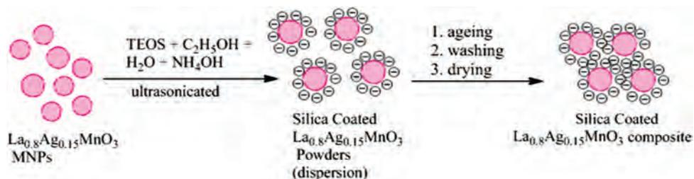
Fig. 1. Schematic of silica coating on  $\text{La}_{0.8}\text{Ag}_{0.15}\text{MnO}_3$  MNPs.
