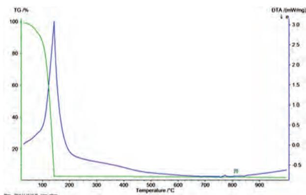
Fig. 4. TG-DTA curves of silica coated LAMO powders.
