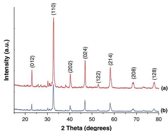
Fig. 2. XRD patterns of (a) bare and (b) silica coated nanocrystalline LAMO powders.
