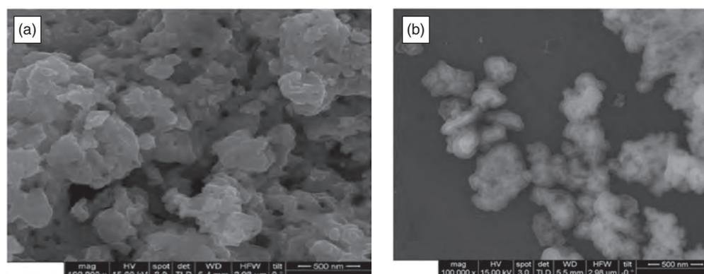
Fig. 3. FE-SEM images of LAMO powders (a) bare (b) silica coated.
