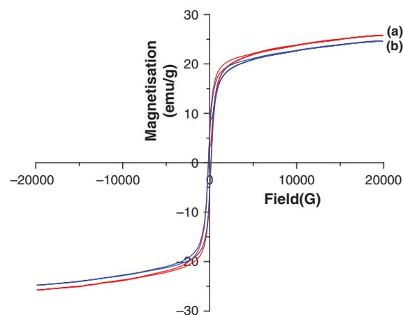
Fig. 5. Magnetic hysteresis curves of LAMO for (a) the bare sample (b) silica coated sample.
