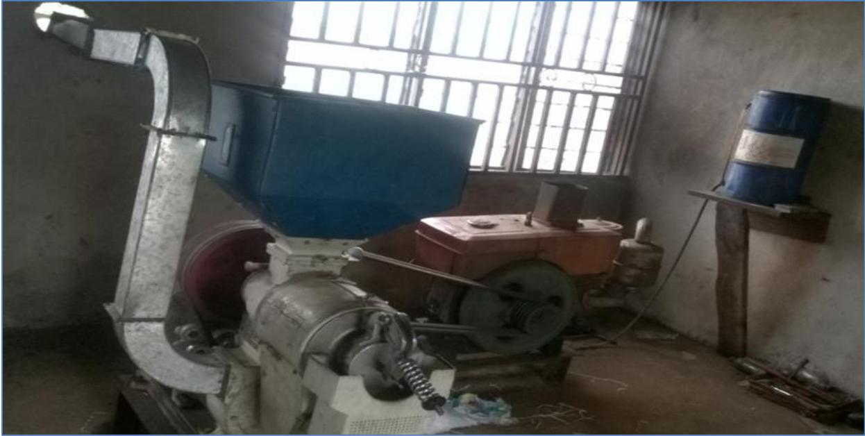
**Figure A3: Stone Removal Machine (*Destoner*)**
