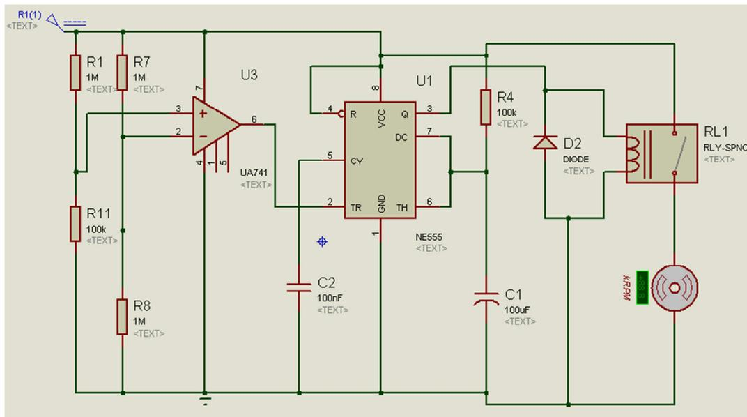
Figure 3.1: The sensing and control circuits
