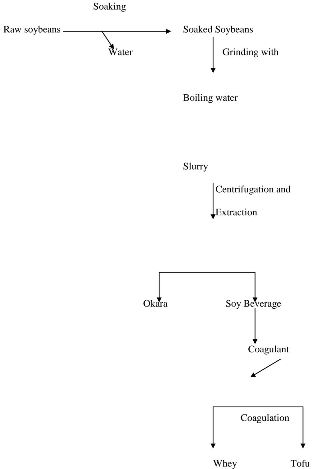
**FIGURE 1: PRODUCTION CHART OF TOFU SAMPLE ANALYSIS**
